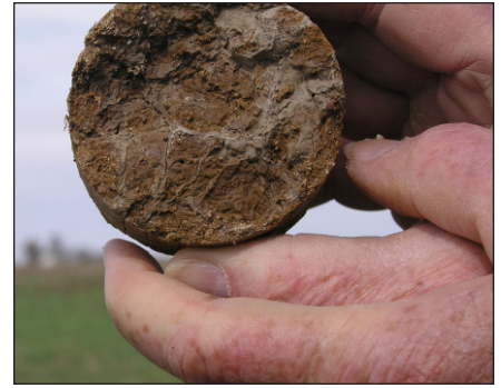
Figure 2. Cross section of the fragipan. The dark brownish areas are cemented and restrict root penetration or water movement.
