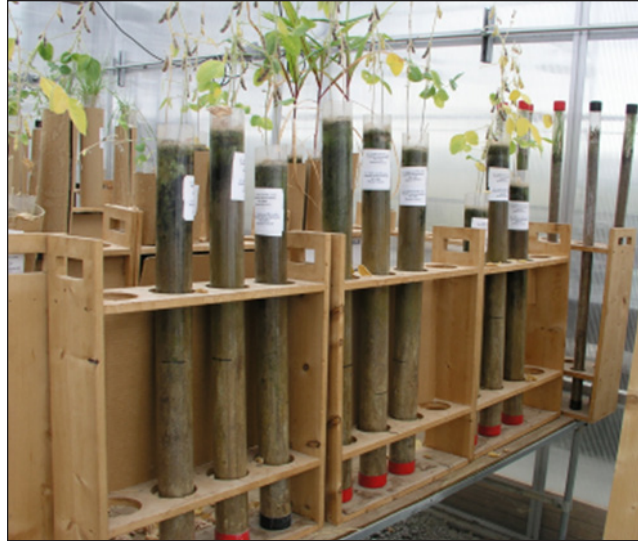
Figure 8. Complete soil profiles in transparent tubes allow for visual verification of different treatments added to break apart the fragipan.
