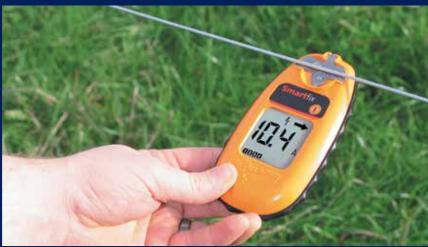
**Use fault finder to monitor voltage and find shorts.** For electric fencing to work properly, a voltage of approximately 5000 volts should be maintained at all times. Shorts in electric fences can cause reduced voltage and can often be difficult to find. A fault finder shows the direction and severity of the of the short. Purchasing a high-quality fault finder is money well spent!
