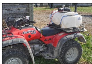
Inexpensive sprayers can be attached to ATVs or golf carts to apply herbicides on small pastures.
